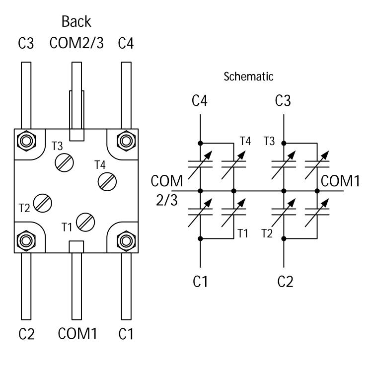
C1 - 5pF to 135pFT1 - 1pF to 10pFC2 - 5pF to 135pFT2 - 1pF to 10pFC3 - 5pF to 25pFT3 - 1pF to 10pFC4 - 5pF to 25pFT4 - 1pF to 10pF
