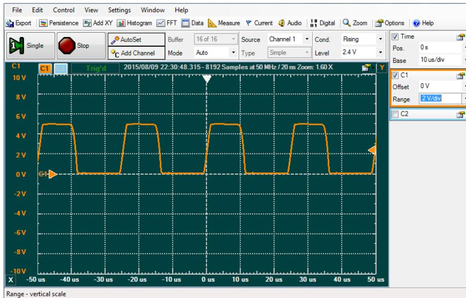
If the Oscilloscope does not display the indicated image, replace XT1 and RT1 and repeat Step 14.
