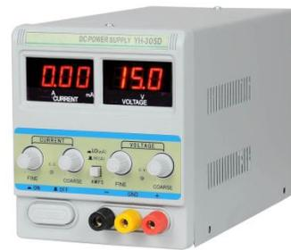
The DC variable power supply can be substituted with the 5V power output pin of the microprocessor system (Arduino, Raspberry Pi, etc.) to be used with the Ultrasonic Range Finder. An old 5V power adaptor can also be used as long as the positive and negative leads are identified before connecting it to the Range Finder board.
