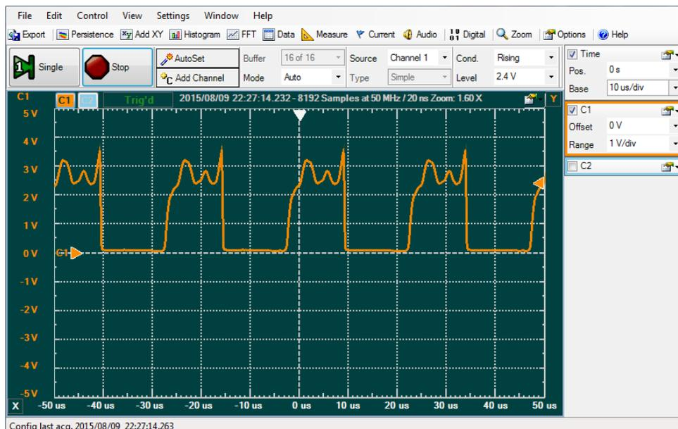
If the Oscilloscope does not display the indicated image, confirm all solder joints to R3, R7, Q2, and U1 Pin 3. Re-solder each pin and repeat Step 8. If re-soldering fails to fix the problem, replace Q2 and repeat Step 8.
