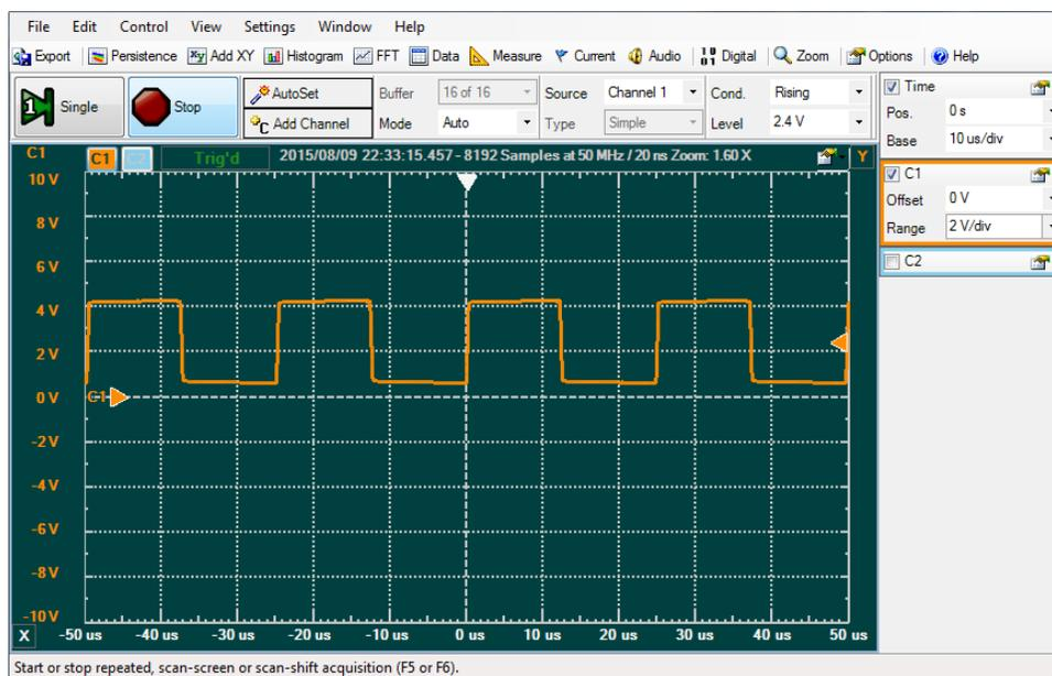
If the Oscilloscope does not display the indicated image, verify all solder joints at U3 Pin 5, U3 Pin 6, U3 Pin 7, C10, and R20. Re-solder each pin and repeat Step 13. If U3 Pin 5 still does not have the signal expected, replace U3.
