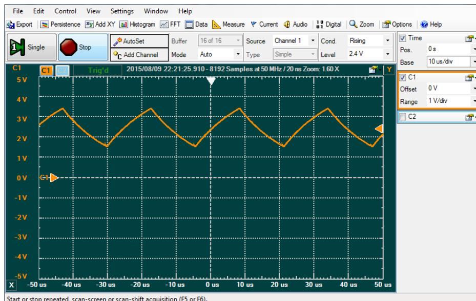
If the Oscilloscope does not display the indicated image, confirm all solder joints to R4, R5, R6, C2, and U1. Re-solder each pin and repeat Step 7. If re-soldering fails to fix the problem, replace U1 and repeat Step 3 through 7.
