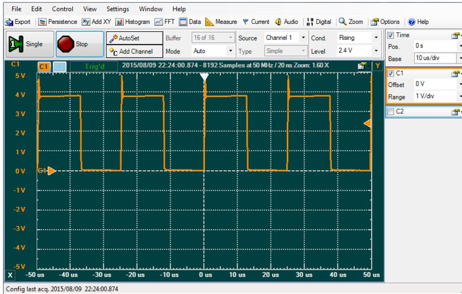
If the Oscilloscope does not display the indicated image, replace U1 and repeat Step 3 through 8.
