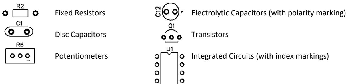
Group components by type and value so that it will be easy to identify them during each assembly step. Straighten all resistor, capacitor, transistor, and potentiometer leads. Kinks and twists in component leads may make it difficult to insert parts onto the PCB.
