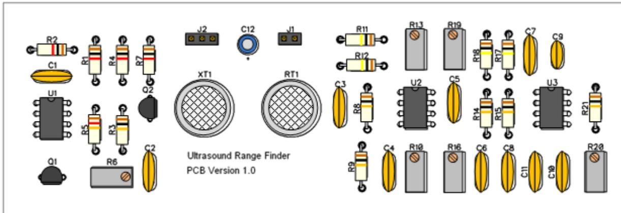
Congratulations on successfully completing the assembly of the Ultrasound Range Finder board! The receiver circuit was designed to allow the builder to adjust the gain and output offsets for different receiver configurations. Before the Range Finder can be used, the transmitter and receiver circuits need to be tested and tuned for the correct frequency, gain, and offset parameters. Follow the procedure steps below to get the Ultrasound Range Finder ready for operation.
