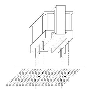
3. ( ) Mount the transformer T1, as shown in the drawing above. Install the transformer in the location indicated in pictorial diagram.
